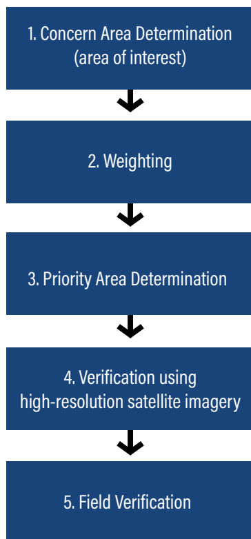
Figure 12 | Stages of Peatland Clearing Monitoring Method
