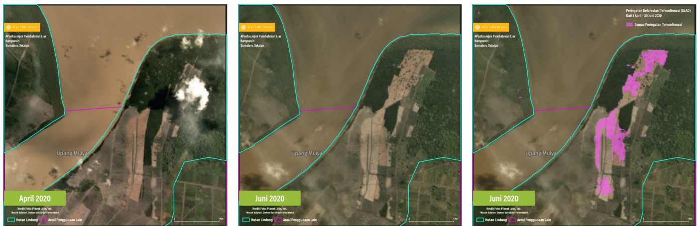
Figure 3 | Example of forest cover change verification using high-resolution satellite images (Planet)
